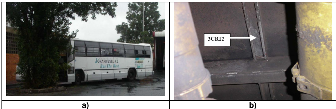
Figure 3.13: a) TFM Bus in 2004, b) View of 3CR12 framework underneath bus. approximately 10 years old (NN 2007).
