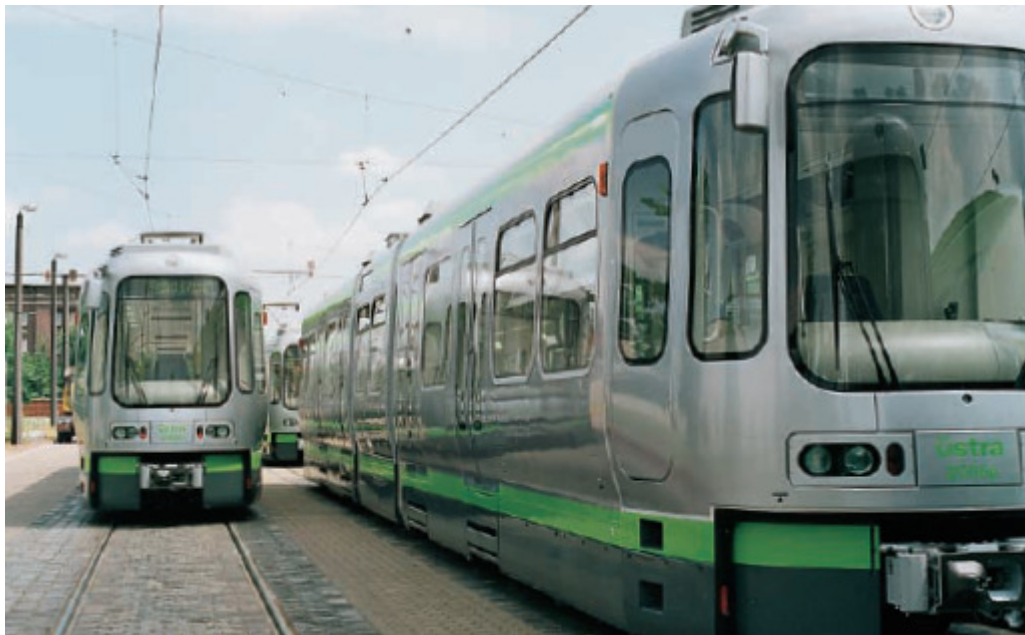
Figure 3.19: Trams built with 3Cr12 frame and bodywork (NN 2004b).
