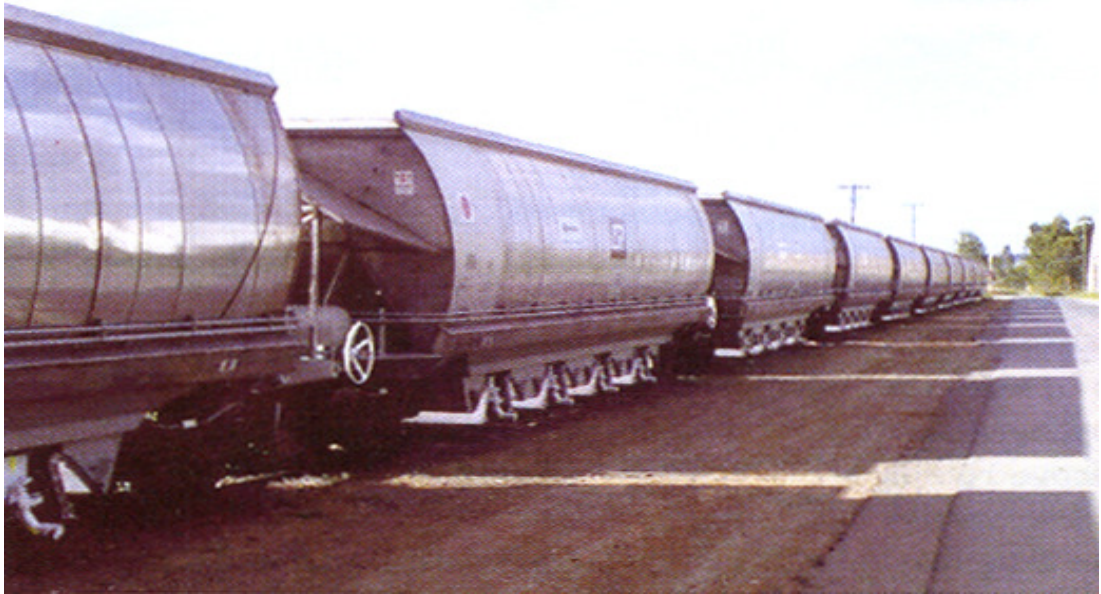
Figure 3.10: Coal wagons for Q-rail, Queensland rail company, the subject of a A$40M order for stainless steel plate and coil and welding wire (NN, 2001).
