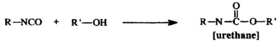
Fig. 1.3. The schematic of reaction with diisocyanate and [-OH][35]
