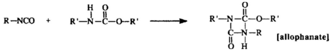
Fig. 1.4. The schematic of reaction with diisocyanate and polyurethane [35]
