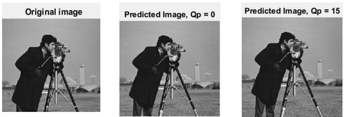
Figure 4.12. Original and predicted frames with Quantization Parameters 0, and 15 using 4x4 Luma Intra Prediction
