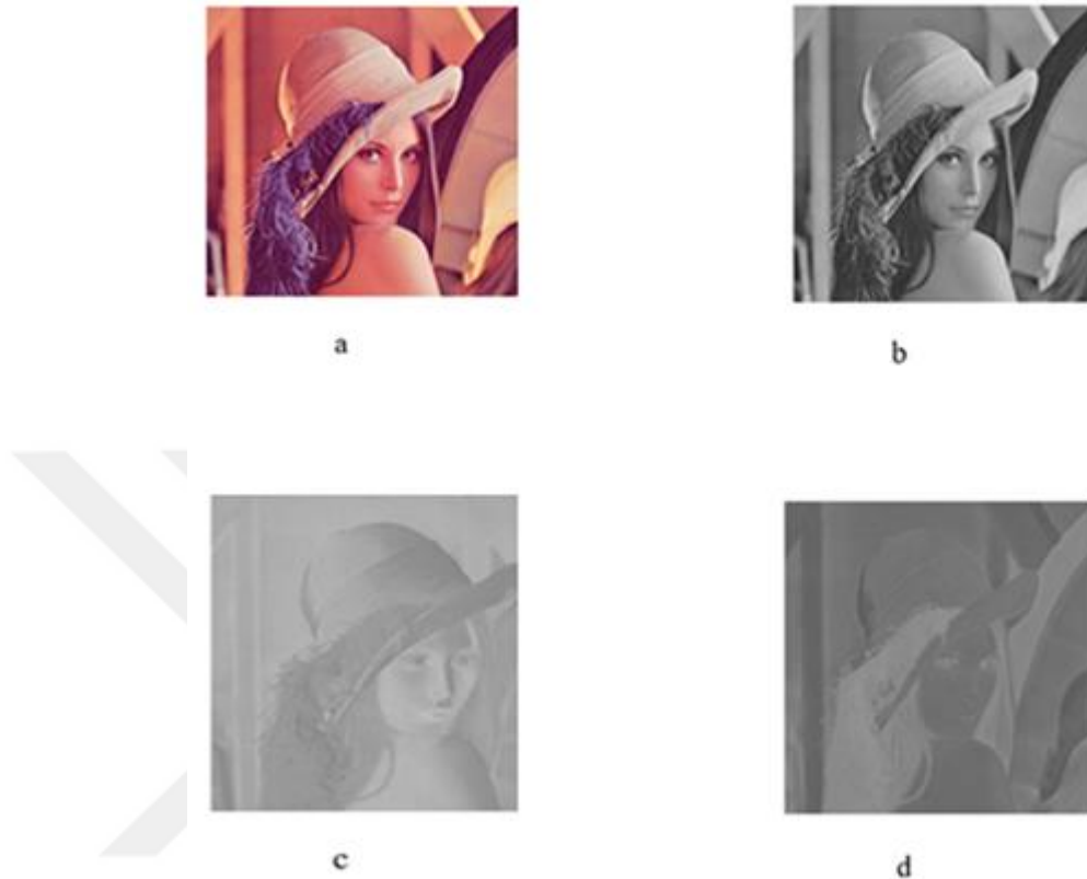
Figure 1.1. A representation of the YCbCr standard. a) The original Photo b) The Y or Luma component of the Photo c) The Cr (Red Chroma) component of the photo d) The Cb(Blue Chroma) component of the photo.
