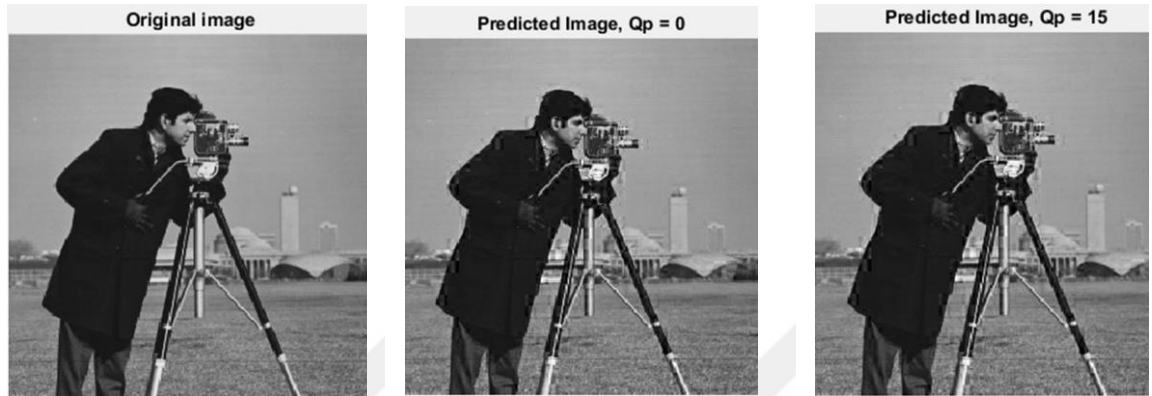
Figure 4.11. Original and predicted frames with Quantization Parameters 0, and 15 using 8x8 Luma Intra prediction
