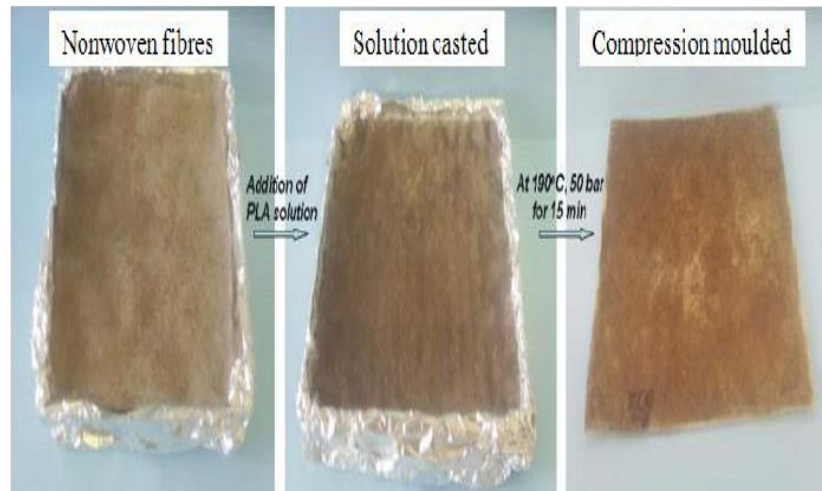
Figure 1. 18. Procedures for preparation of nonwoven PLA composites [185]
