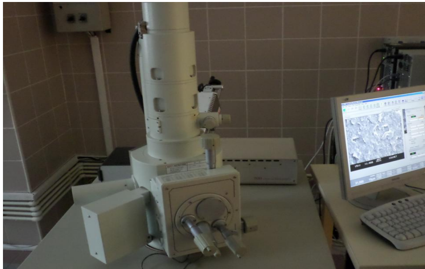
Figure 2. 25. Edwards coating system, E306A, USA (a), Scanning Electron Microscope, Philips XL30 (b)
