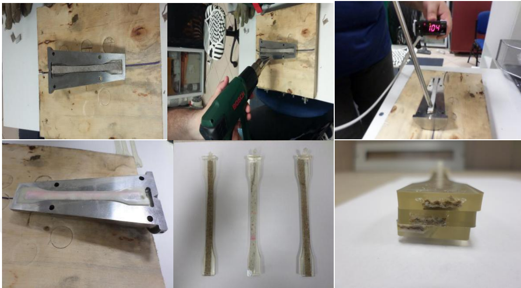
Figure 2. 7. Preparation of the PLA/JUTE in photos
