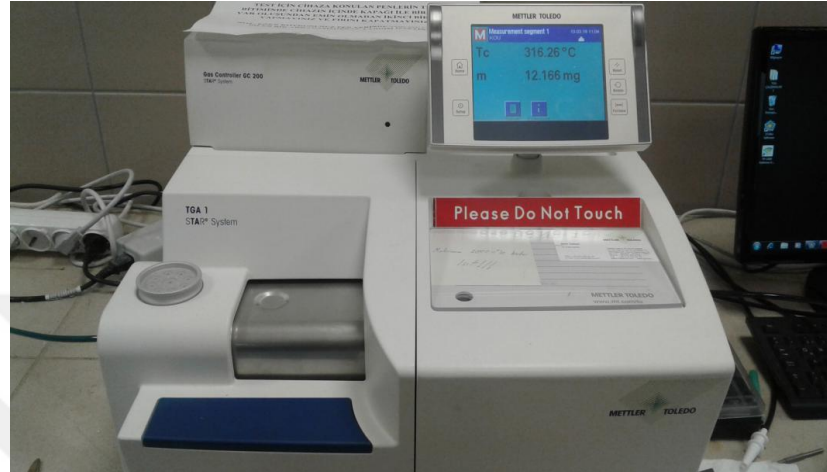
Figure 2. 23. Thermogravimetric analysis 3-TGA used in measuring thermal characteristics of sample
