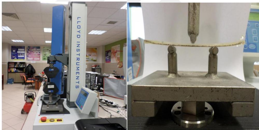
Figure 2. 15. Composite specimen undergoing flexure testing
