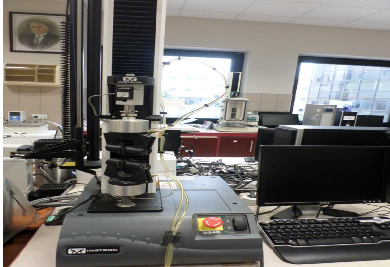
Figure 2. 12. Composite specimen tensile testing
