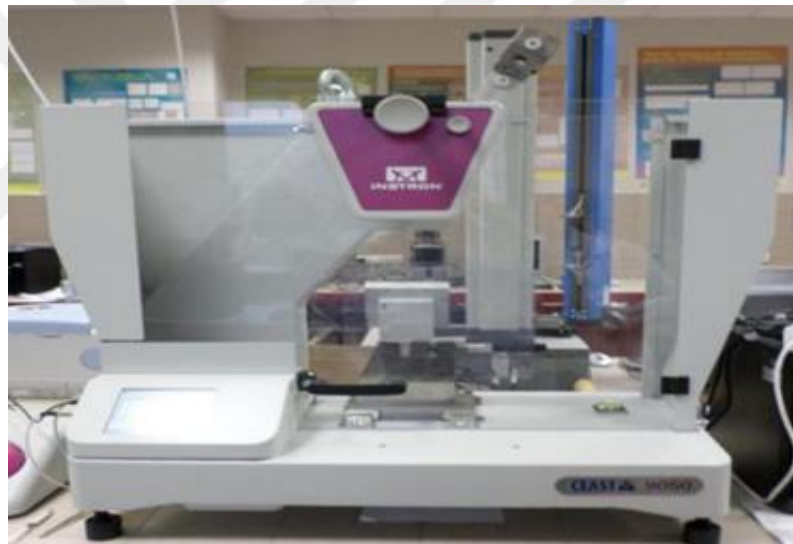
Figure 2. 17. Composite specimen undergoing impact testing
