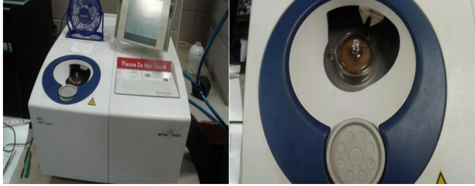
Figure 2. 21. Differential scanning calorimetry – METTLER 2 DSC used in measuring thermal characteristics of sample
