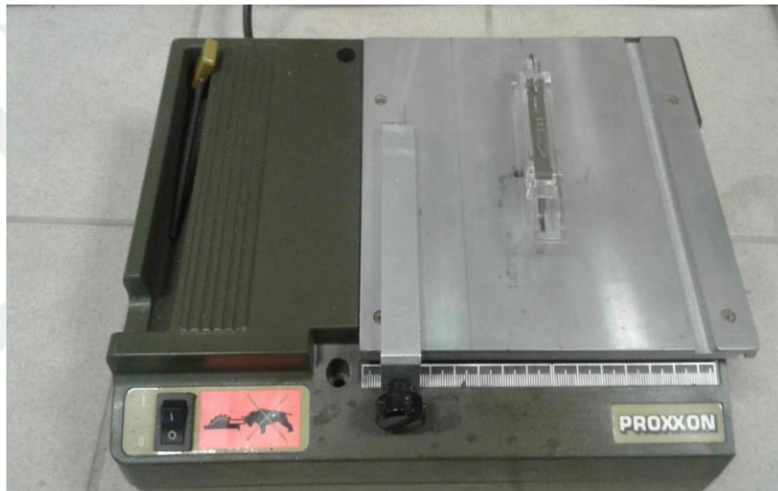
Figure 2. 11. Bench Circular Saw
