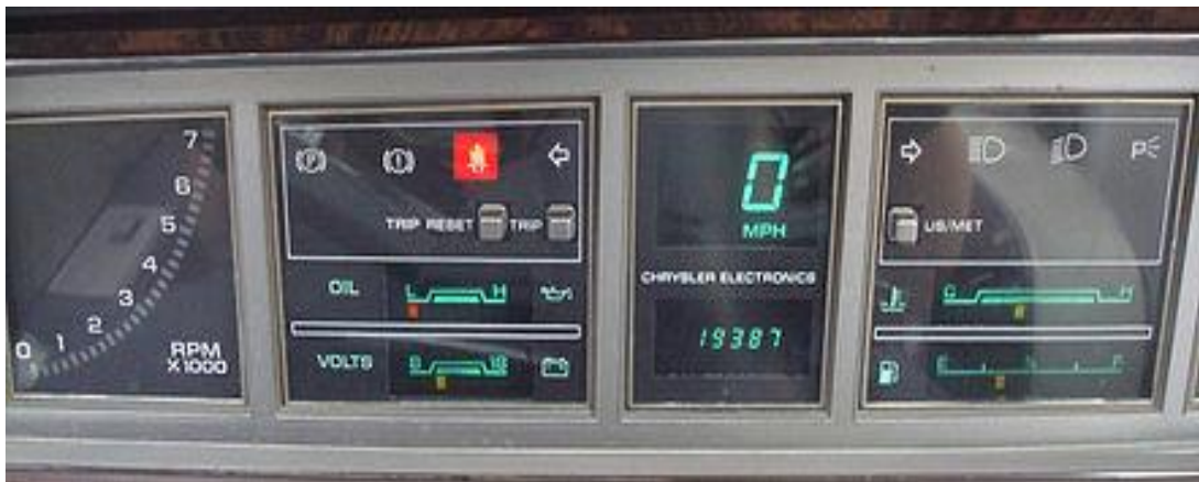
Figure 1.8. Digital instrument cluster from the 1984 Dodge 600 [14]
