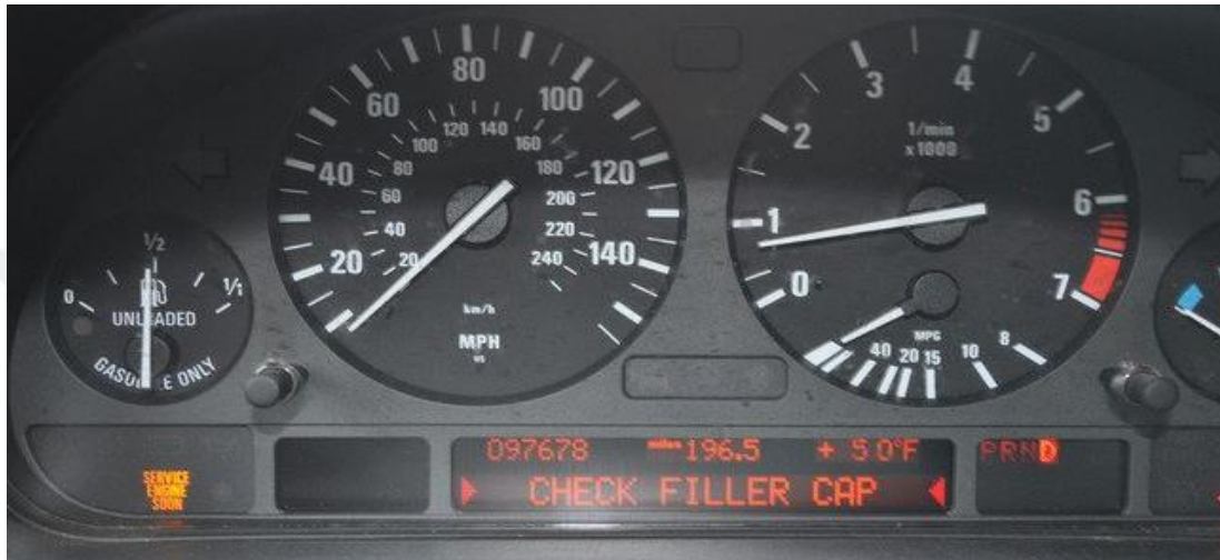
Figure 1.9. “CHECK FILLER CAP” warning on BMW E39 character display [15]
