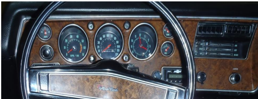
Figure 1.7. Analog instrument cluster in the 1971 Chevrolet Monte Carlo [13]
