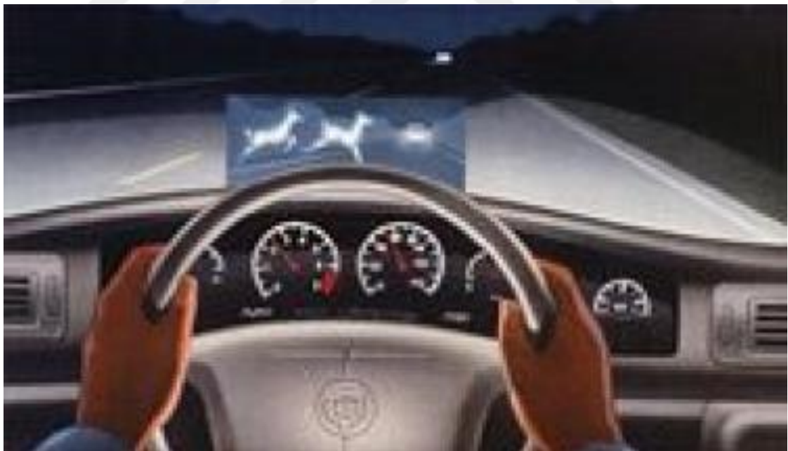
Figure 1.5. Night vision enhancement system [11]
