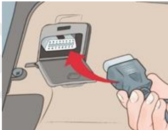
Figure 2.7. Standard OBD-II Connector [23]
