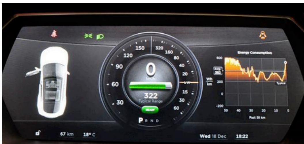
Figure 1.10. Virtual Instrument Cluster in Tesla Model S [16]
