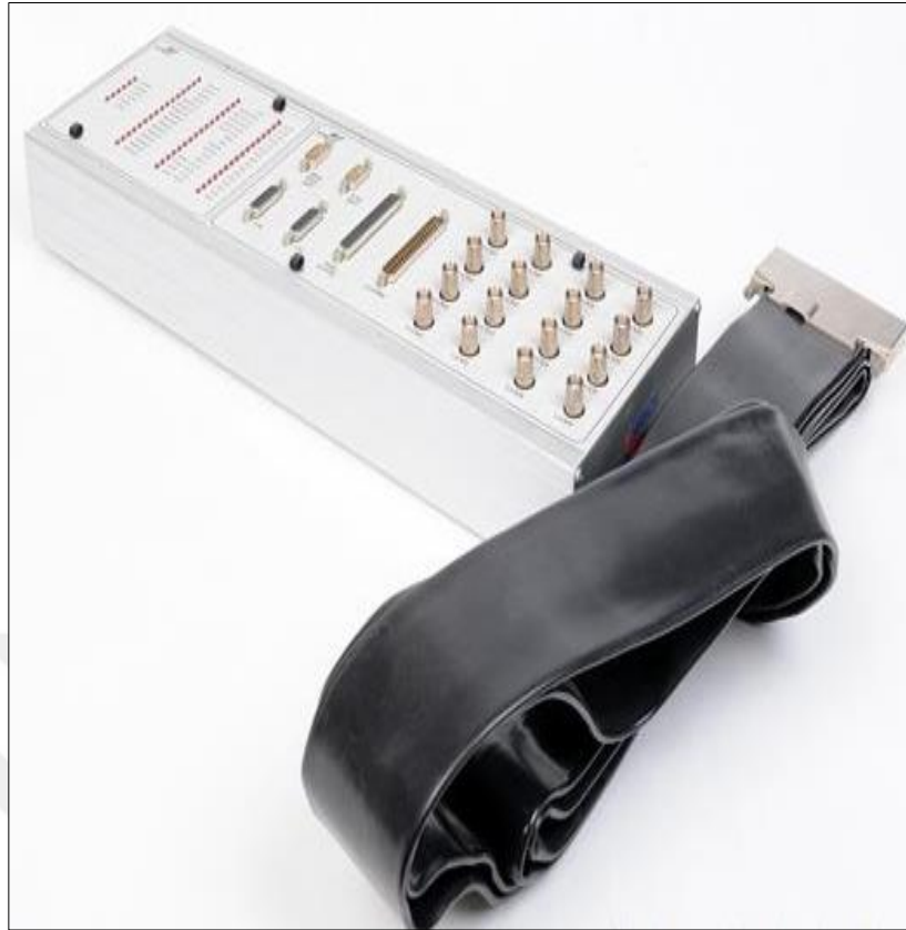
Figure 5.6. An example of a dSPACE controller board
