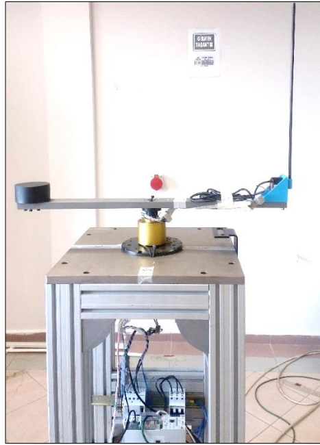
Figure 5.7. Real experimental implementation of the SLRIP
