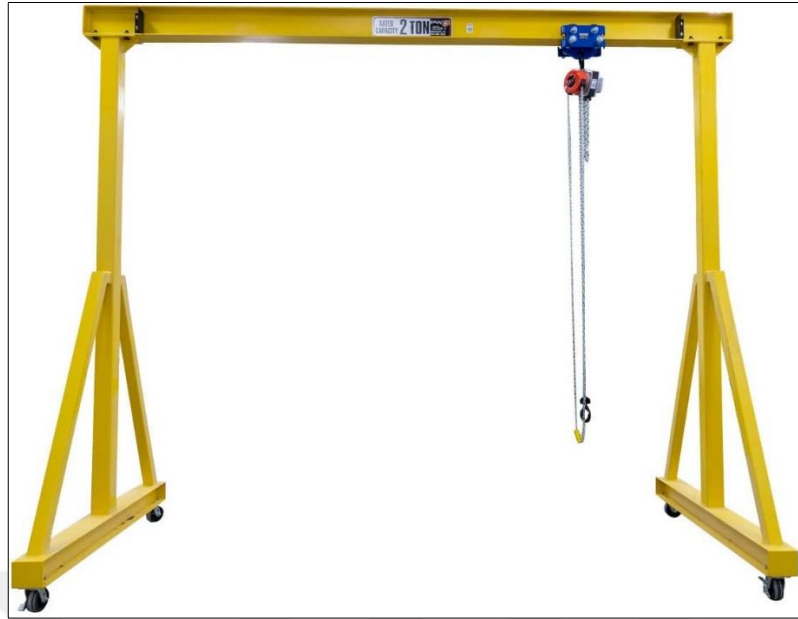
Figure 1.25. Example of a gantry crane system
