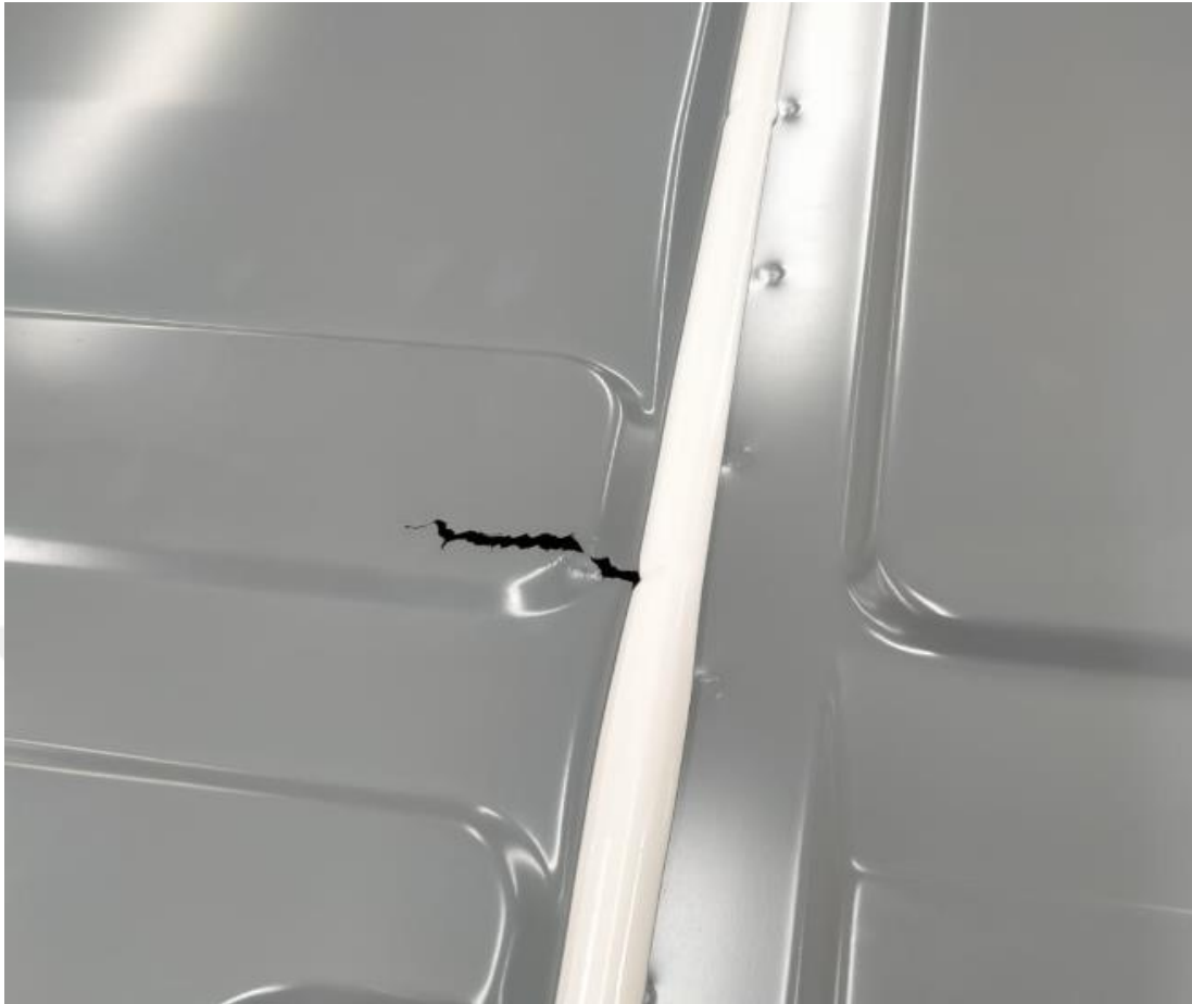
Figure 7. 7.Large Dimension Sheet Metal Part Split Issue
