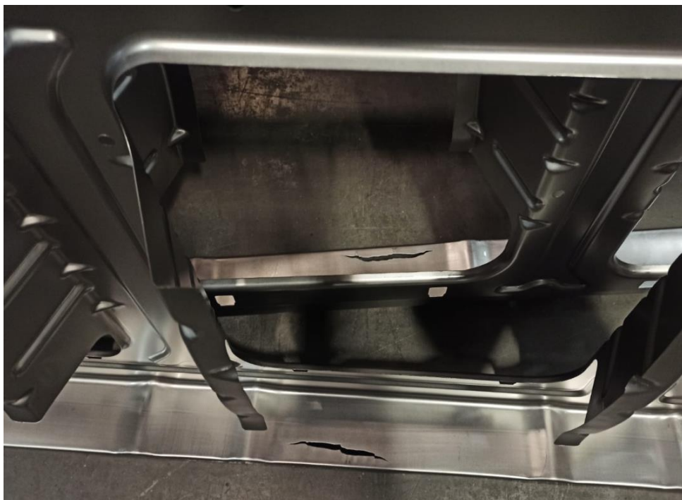
Figure 7. 6.Sheet Metal Split Issue
