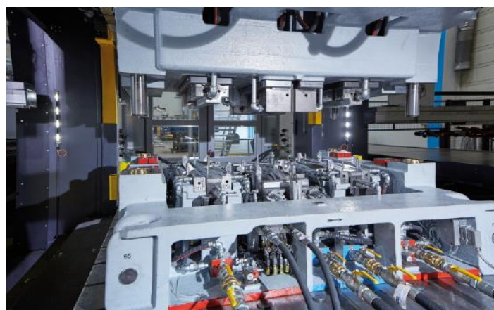
Figure 7. 23.Cooling Pipe System in Hot Stamping [5]
