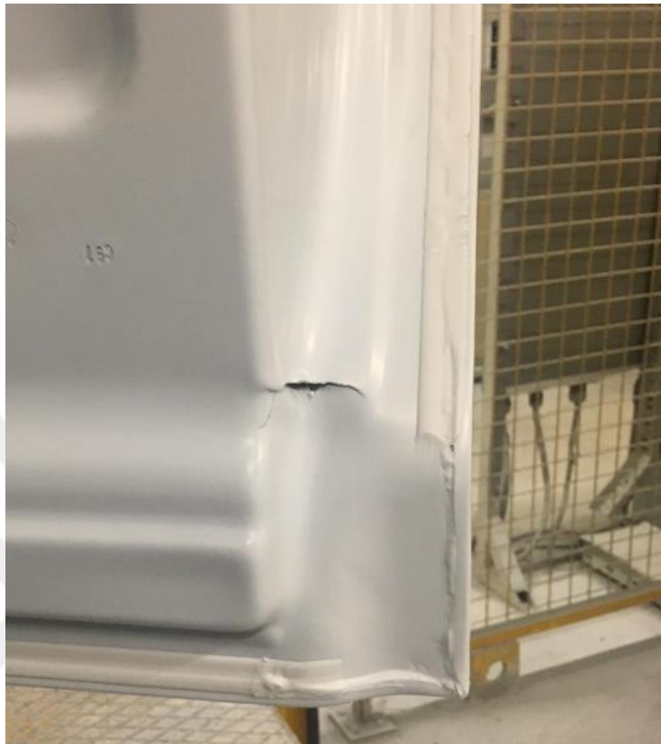
Figure 7. 5.Sheet Metal Inner Part Split Issue
