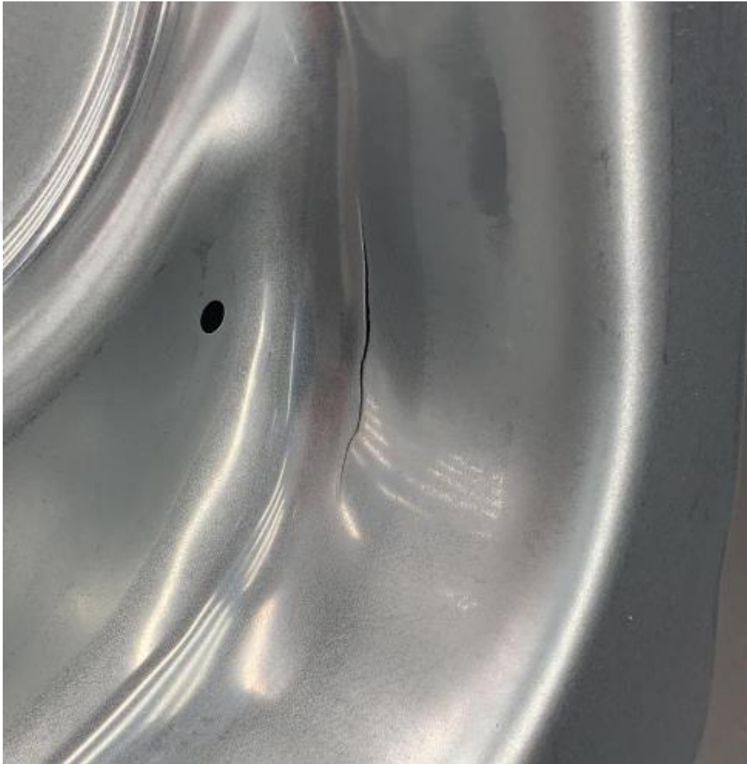
Figure 6. 8.Wall Split Issue in Mass Production in 12 SPM
