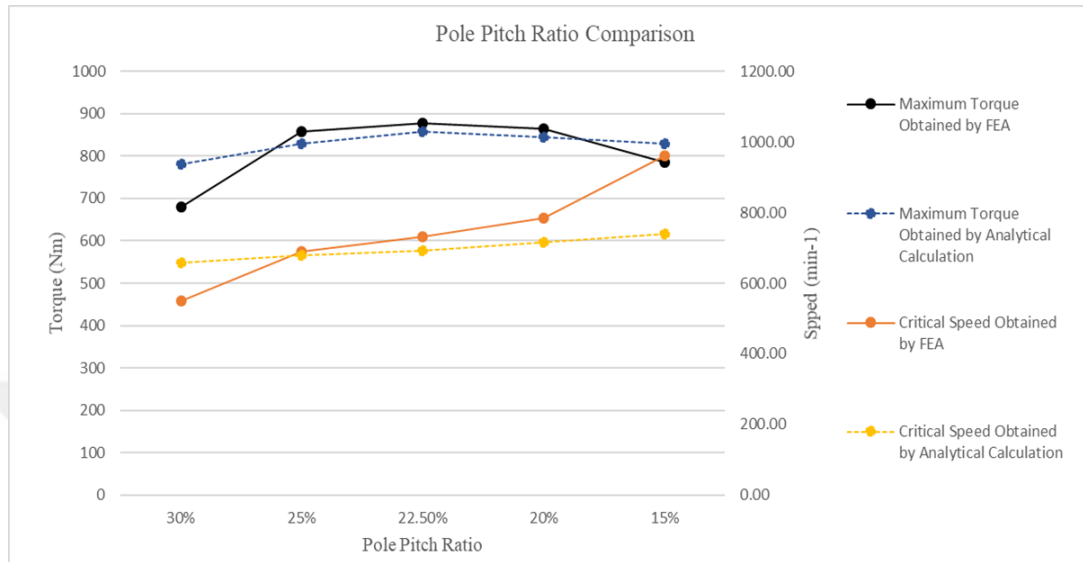
Figure 3.6. Maximum torque and critical speed values of different pole pitch ratios
