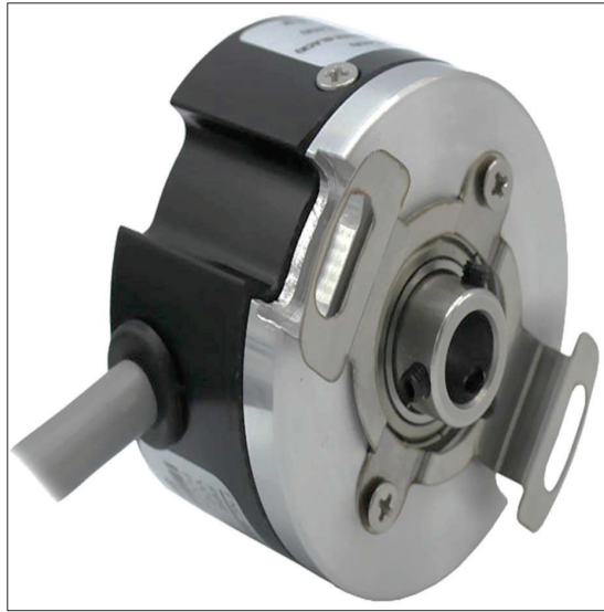
Figure 5.4. Encoder (Model: Fenac, Type: 2048 PPR sin cosine accurate speed information)
